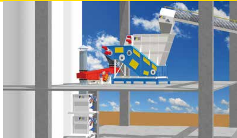
Integration in the preheater tower (PHT): Doseahorse, vibrating conveyor and electrical double valve airlock
