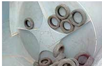
Singulator: extractor for whole tyres
