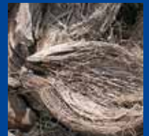
Coconuts shells 50 - 250 mm d = 0,25 t/m³
