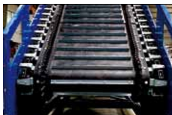
Metallic apron with rubber belt sealing
